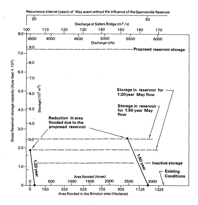
the natural waterway through the Brinston area. The effects of channelization were accounted for by shifting the stage/-flooded area relationship to reflect the new threshold of flooding at  $102 \text{ m}^3/\text{s}$  (3600 cfs).
