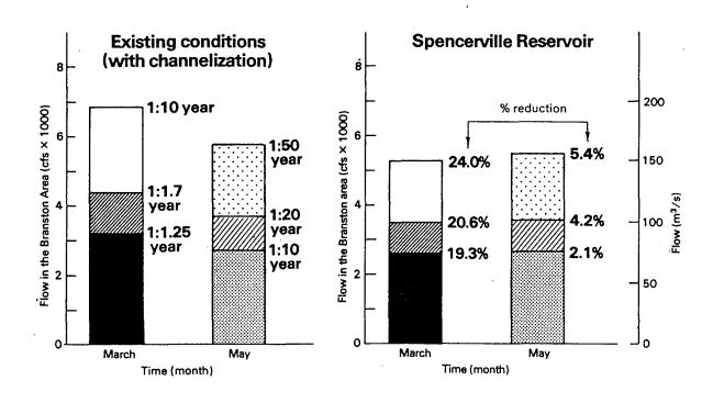
tions revealed that the reservoir is only partially filled during flood conditions. Twenty percent of the live storage was used during the 50 year event with progressively smaller storage volumes retained during less severe flood discharges.
